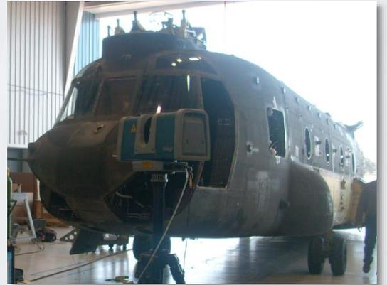
*EMS 3D scanned much of the exterior with the Surphaser long range scanner.*
