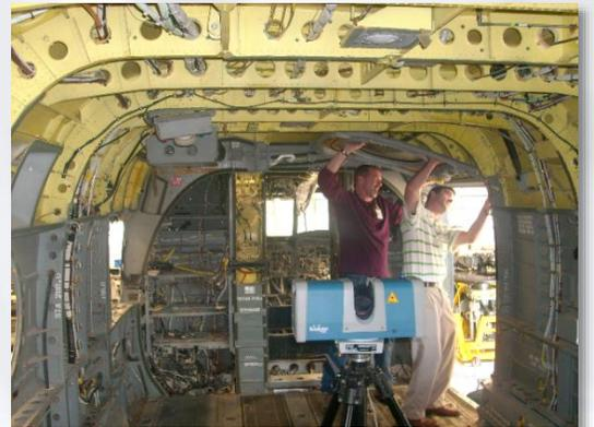
*EMS used multiple 3D scanners for the interior.*
