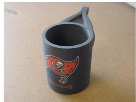
3D Printed Model in Full 3D Color using a Z Corp Z650 3D Printer
