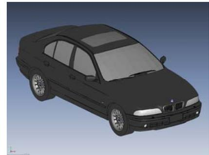
Finished CAD model from 3D scan data
