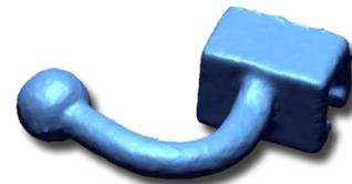
Raw scan of part with .018 mm point spacing
