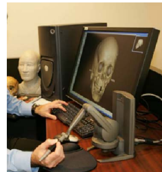
Using SensAble to 3D sculpt a face over the 3D scan data of the skull
