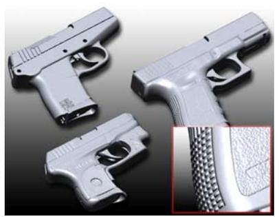
Numerous sample CAD models from scan data. Inset shows detail in grip area
